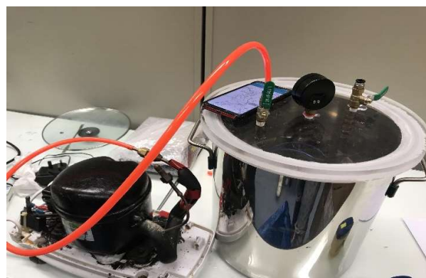
Figure 2. Device for Accelerating the Evaporation of a Brine Solution
