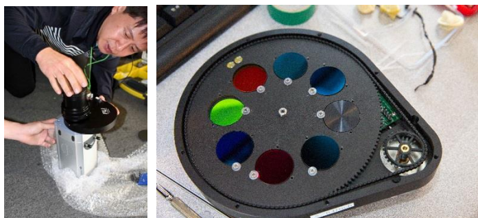
Figure 4 - Astronomical CCD camera and filter wheel of CQUEAN (Park et al. 2012, Publications of Astronomical Society of the Pacific, 124, 839).
